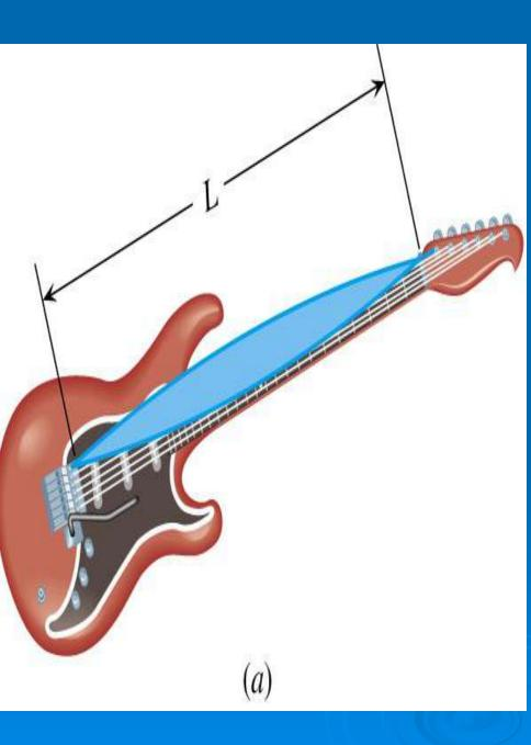
The heaviest string on an electric guitar has a linear density of 5.28 X 10<sup>-3</sup> kg/m and is stretched w/a tension of 226N. This string produces the musical note E when vibrating along its entire length in a standing wave at the fundamental frequency of 164.8 Hz. Find the length L of the string between its two
