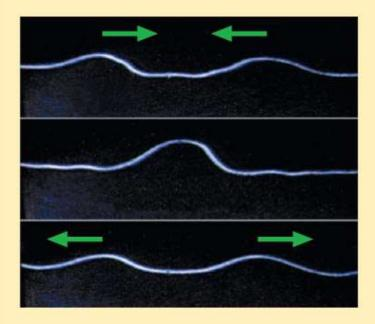
Two waves on a string each displace the string upward. Where the two waves overlap, the displacement is twice that of the individual waves. This is **constructive interference.**
