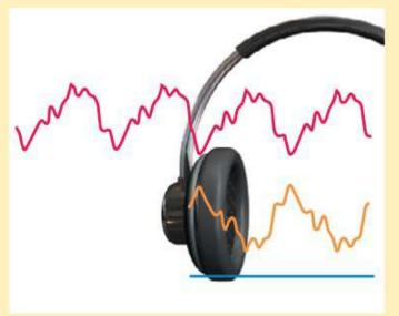
Noise-canceling headphones create a sound wave that is inverted from the ambient sound. When the waves are added, they cancel, producing a much smaller wave. This is **destructive interference.**
