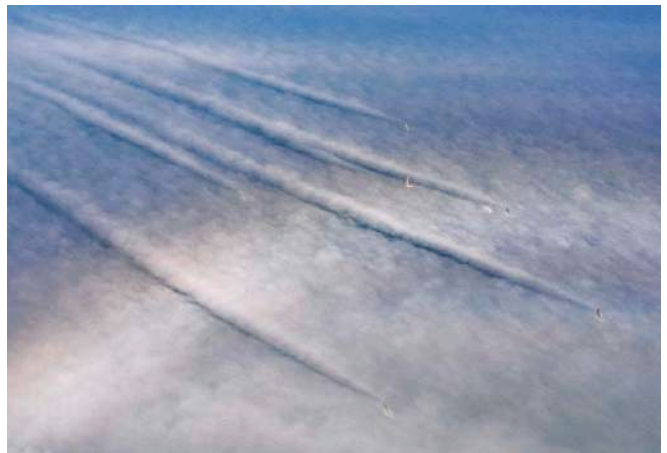
FIG. 11: Tip vortices, a form of lift-induced drag, created by the sails of yachts sailing on a close haul, made visible by the fog during the 2001-2003 Volvo Ocean Race. Photo by Daniel Forster, taken from Ref. [20].
