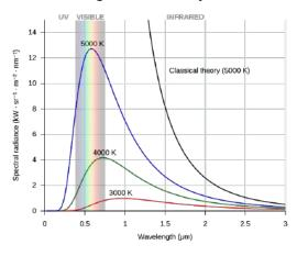
Spectrum of thermal radiation: "ultraviolet catastrophe"
