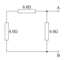
Calculate the total resistance between point A and point B of this arrangement.
