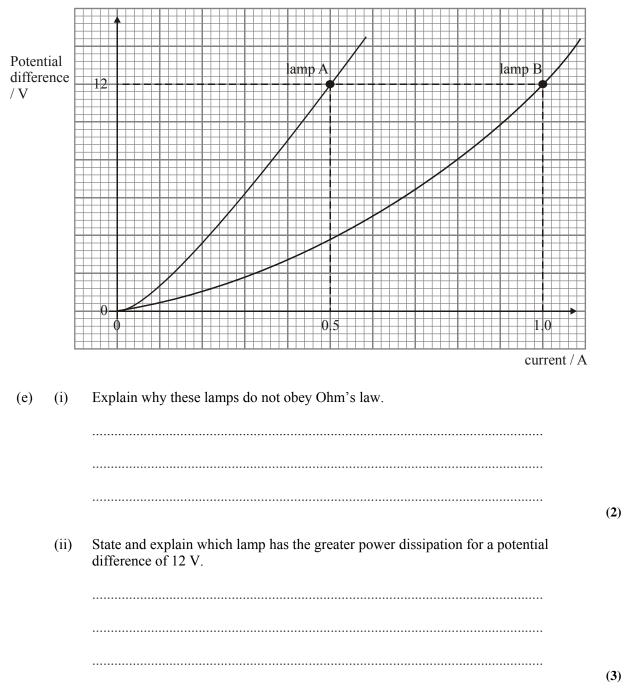
The graph below shows the V-I characteristic for two 12 V filament lamps A and B.
