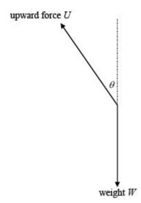
correct relative directions of forces; upward force length greater than weight by eye; appropriate labelling of forces; angle  $\theta$  as shown above; *Award* [2 max] if extra force(s) drawn.
