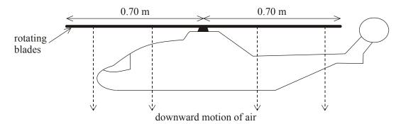
The rotating blades of the helicopter force a column of air to move downwards. Explain how this may enable the helicopter to remain stationary.
