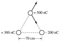
As shown above, the vertical components of the forces subtract and the horizontal components add.
