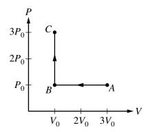
A sealed cylinder with a moveable piston contains N molecules of an ideal gas. The gas is initially in state A shown on the above PV diagram, where P is pressure and V is volume. The gas is then taken through the two processes shown.
