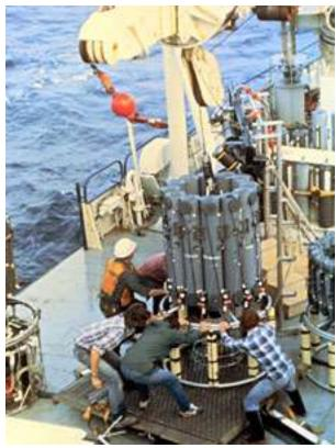
deployed off ship usually; data fed back to ship in realtime Niskin bottles sample ocean water at predetermined depths "casts" can take many hours
