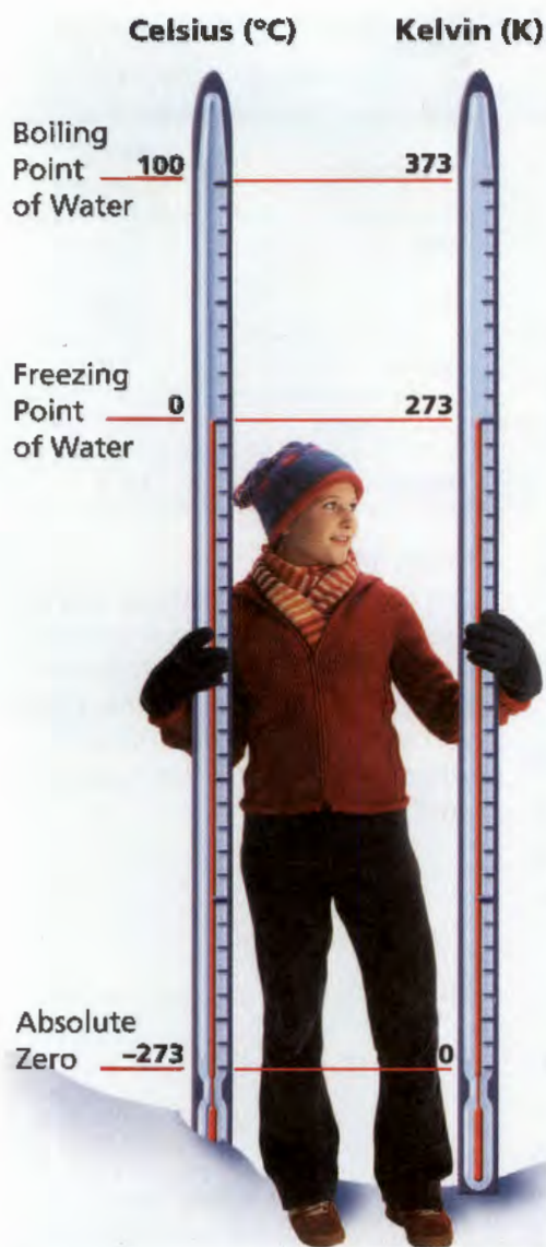
FIGURE 16 Measuring Temperature Scientists use the Celsius and Kelvin scales to measure temperature.
