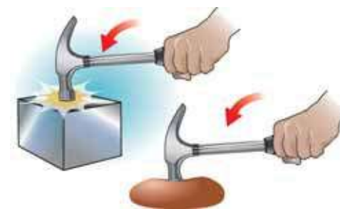
Figure 5.12: Steel and rubber are both solids but they have different strengths, or abilities to hold their shape under force.
