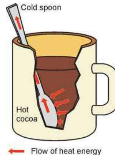
Figure 5.17: Heat flows by conduction from the hot cocoa into the spoon and up its handle.
