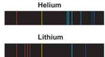
Figure 16.18: Spectral lines for helium and lithium. Each element has its own unique pattern of spectral lines (spectrum).
