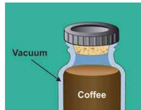
Figure 5.19: A thermos bottle uses a vacuum to prevent heat transfer by conduction or convection.
