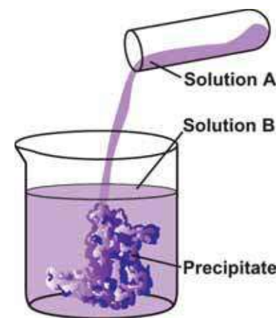
Figure 10.8: The formation of a cloudy precipitate is evidence that a double-displacement reaction has occurred.
