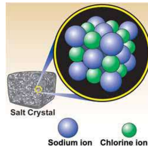
Figure 5.14: The shape of a salt crystal is due to the arrangement of sodium and chlorine atoms at the submicroscopic level.
