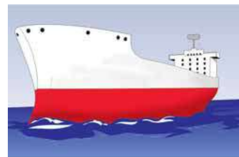
Empty cargo ship - less displaced water
