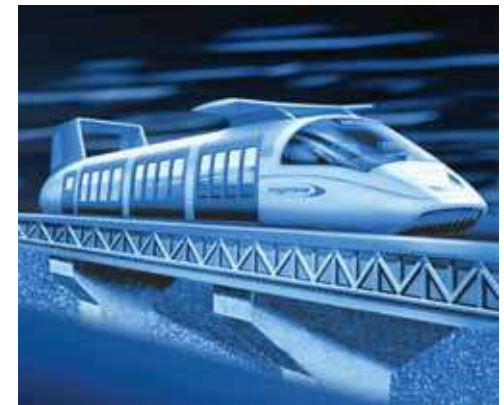
Figure 13.9: With a maglev train, there is no contact between the moving train and the rail — and thus little friction.
