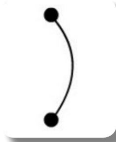
Self-Resetting Circuit Breaker Symbol
