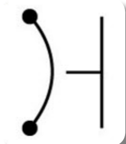
Manually-Resetting Circuit Breaker Symbol
