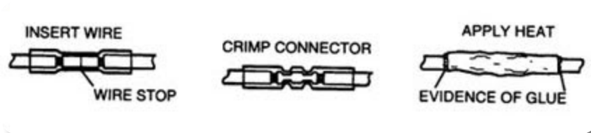
Splice Sleeve Crimping Steps
