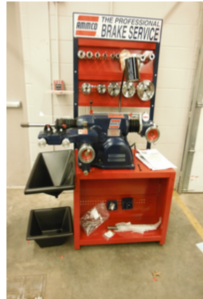
Brake Machine Setup to Turn Rotors
