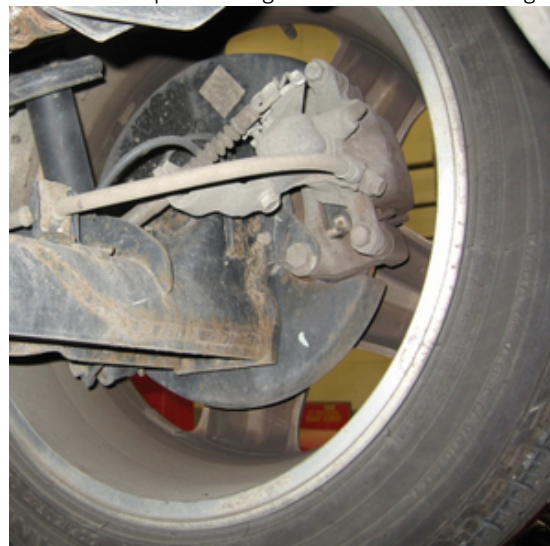
Rear Caliper Parking Brake Cables and Linkage
