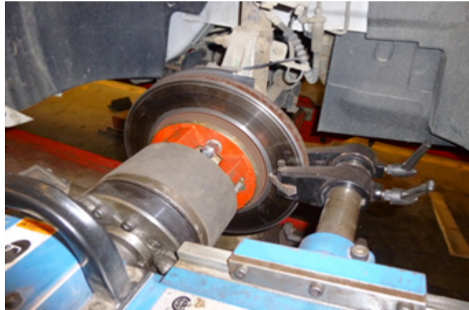
Lathe Just Beginning First Cut. Notice the 'Zero Point' cut near the edge.
