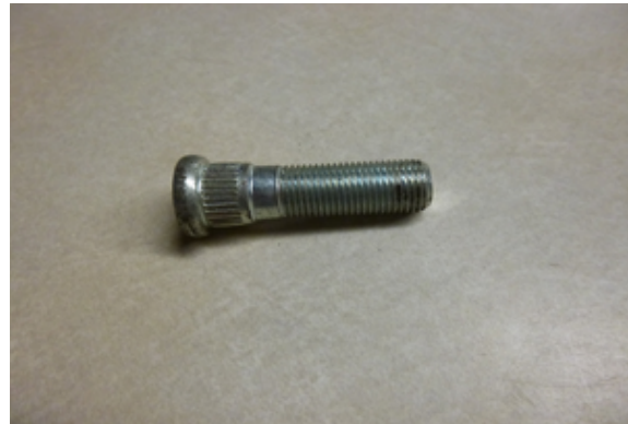
Replacement Wheel Stud
