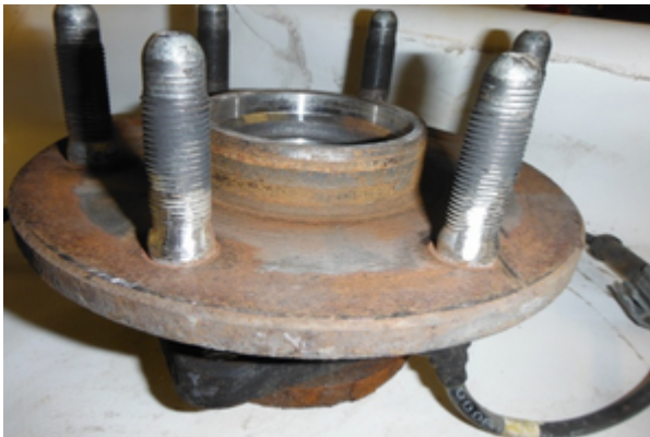
Damaged Wheel Studs
