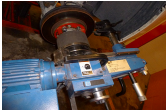
Setting Cutting Bits to 'Zero Point'
