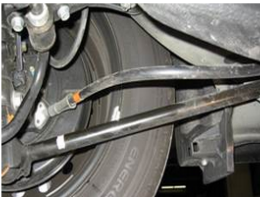
Parking Brake Cable Routing to Rear Brake
