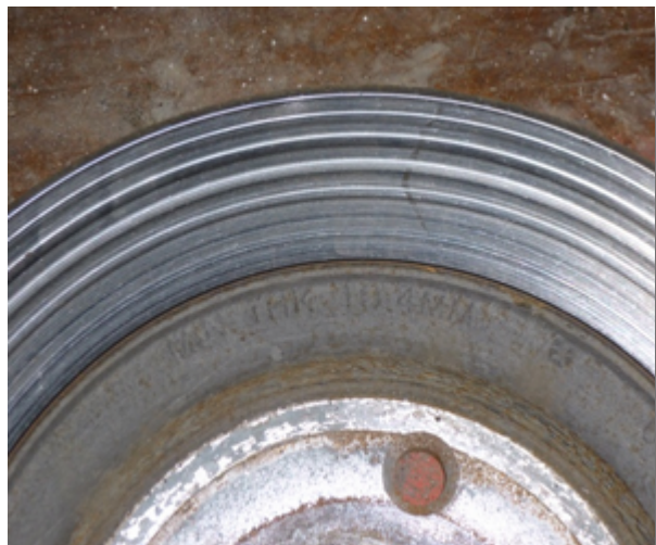
Worn Brake Rotors
