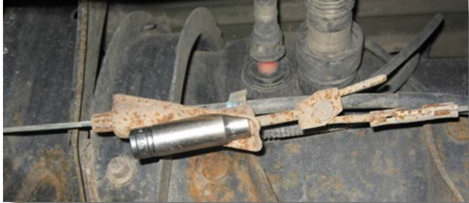
Parking Brake Adjusting (Equalizer) Screw and Nut
