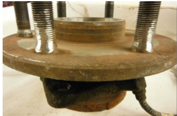
Damaged Wheel Studs
