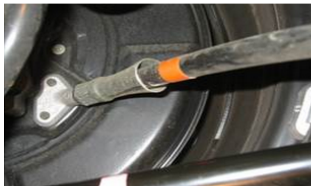
Parking Brake Cable Connection to Rear Brake
