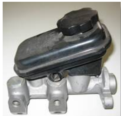
Master Cylinder with Reservoir
