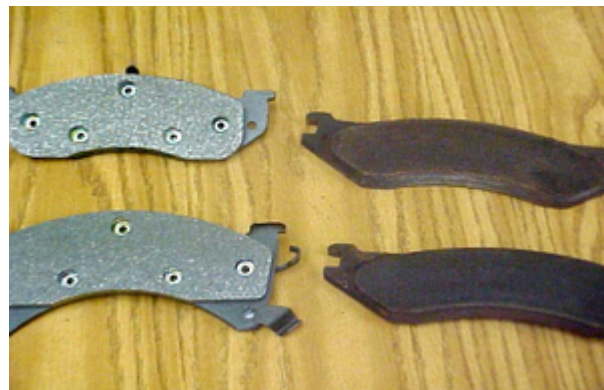
Left-New Brake Pads Right-Used / Damaged Brake Pads
