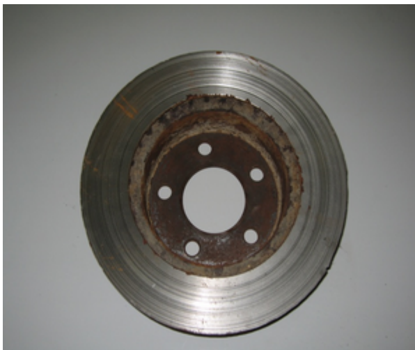
Worn Brake Rotors
