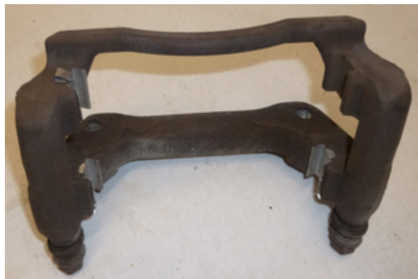
Caliper Mounting Bracket with Guides
