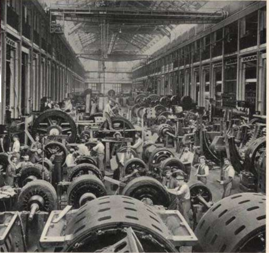
Winding Large Rotating and Stationary Armatures
