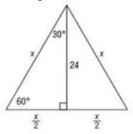
In a 30°-60°-90° triangle, the length of the hypotenuse *h* is 2 times the length of the shorter leg *s* (*h*=2*s*) and the length of the longer leg *l* is  $\sqrt{3}$  times the length of the shorter leg  $(l = s\sqrt{3})$ .
