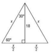
In a 30°-60°-90° triangle, the length of the hypotenuse *h* is 2 times the length of the shorter leg *s* (h=2s) and the length of the longer leg *l* is  $\sqrt{3}$  times the length of the shorter leg  $(l = s\sqrt{3})$ .
