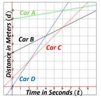
To compare these race cars, we need to know their speeds. The speed is a measure of distance over time, which is the slope or steepness of each line. So let's find the slope for each race car. After finding the rise and run for each car, we should come to the following values:
