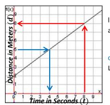
To solve using the graph, simply go to 8 seconds and move up to the line. How far did the car travel? It looks like the toy car has traveled 8 meters at that point.
