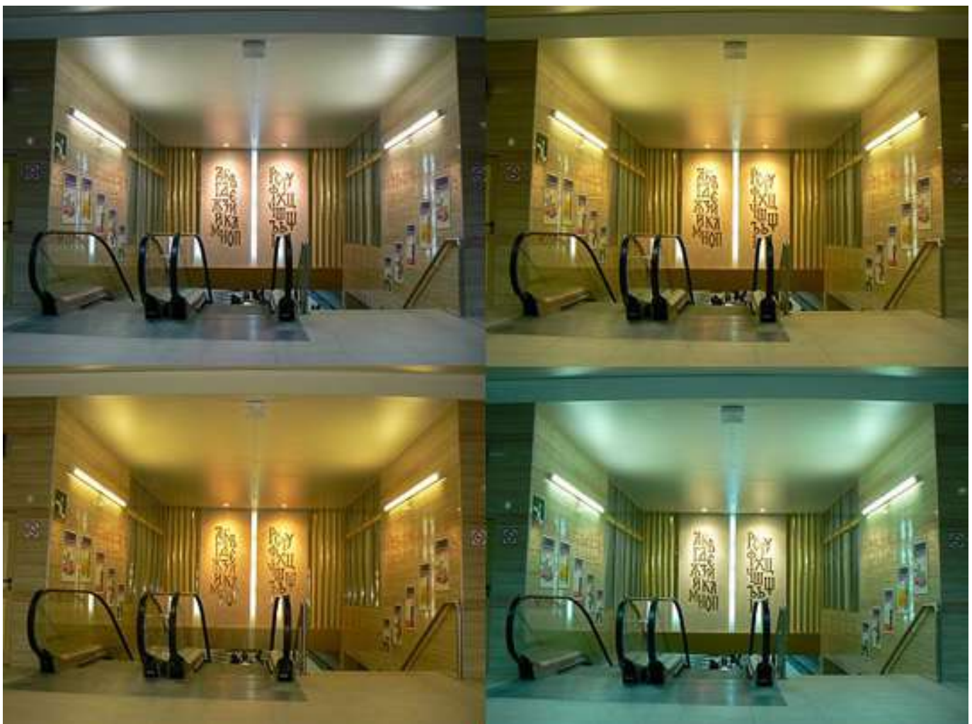
This illustrates the differences in the white balance setting: upper left: auto WB; upper right: sun; lower left: flash; lower right: wolfram bulb
