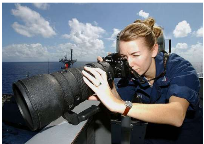
A 400mm fixed telephoto lens being used to photograph daily activity aboard an aircraft carrier.
