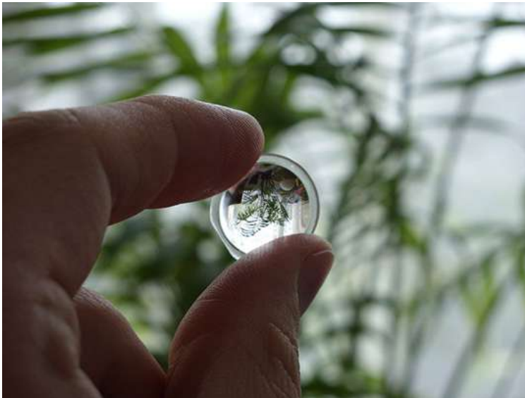
A biconvex lens showing the inverted image.
