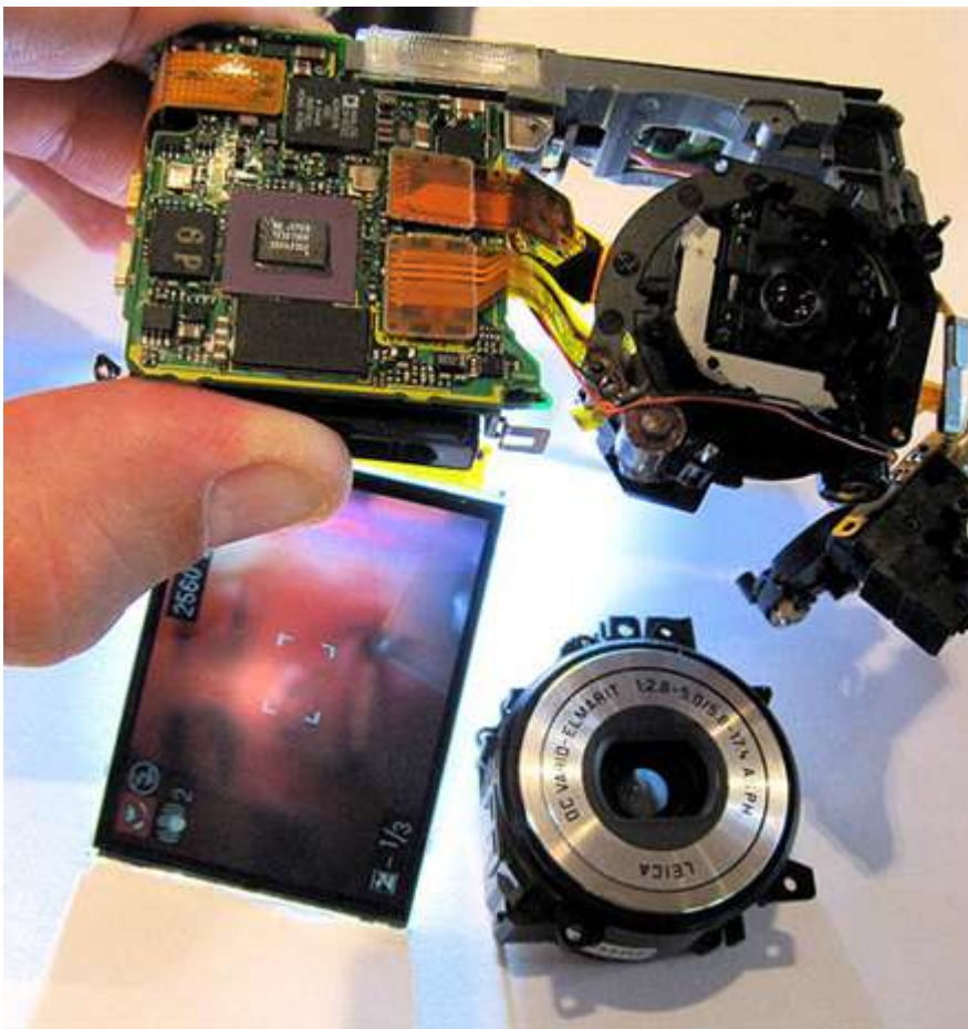
A partly disassembled Panasonic Lumix digital camera, with the front lens removed, but still functioning (see display).
