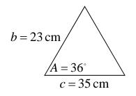
Area =  $\frac{1}{2}bc(\sin A)$ . We use the angle in between the two sides and take the sine of that angle.
