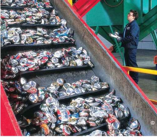
FIGURE 18 Metal Recycling Metal is a commonly recycled material. Here, crumpled aluminum cans ride up a conveyor belt in a recycling center. Predicting Without recycling, what might eventually happen to the supply of aluminum?
