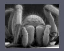
Specimen is sprayed with a fine metal coating then a beam of electrons is passed over the surface
