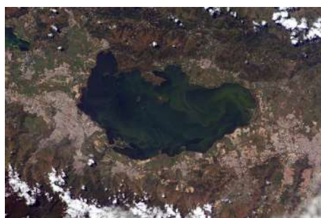
Figure 8.8: Lake Valencia, Venezuela, showing vivid green algal blooms, resulting from continued influx of untreated wastewater from surrounding urban, agricultural, and industrial land uses. This contributes to ongoing eutrophication, contamination, and salinization of the lake. This pollution impacts the lake's use as a reservoir for the surrounding urban centers and limits opportunities for tourism and recreational uses as well.
