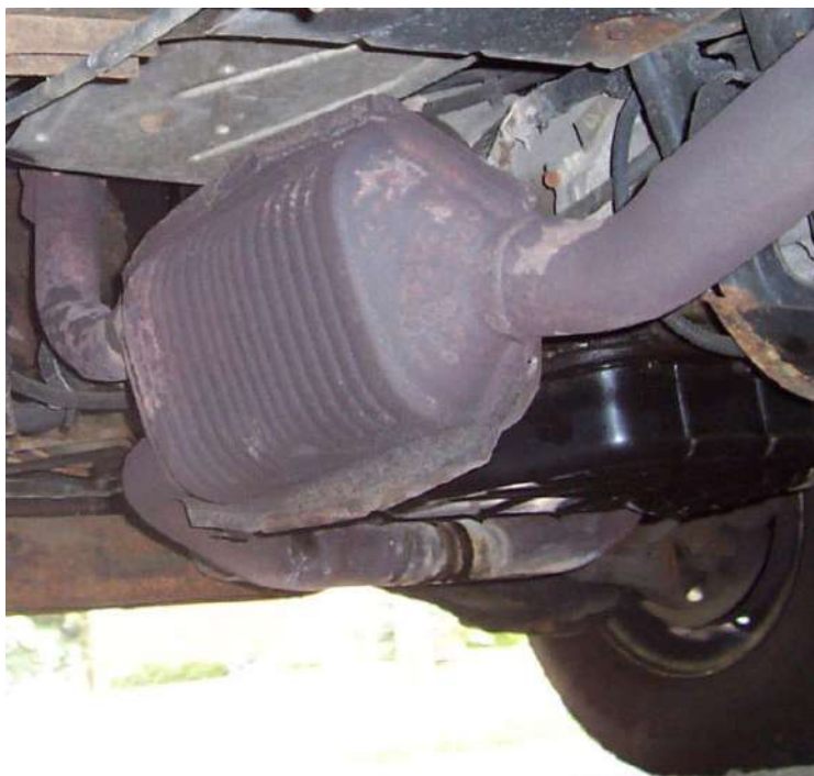
Figure 5.12: A large catalytic converter on an SUV.
