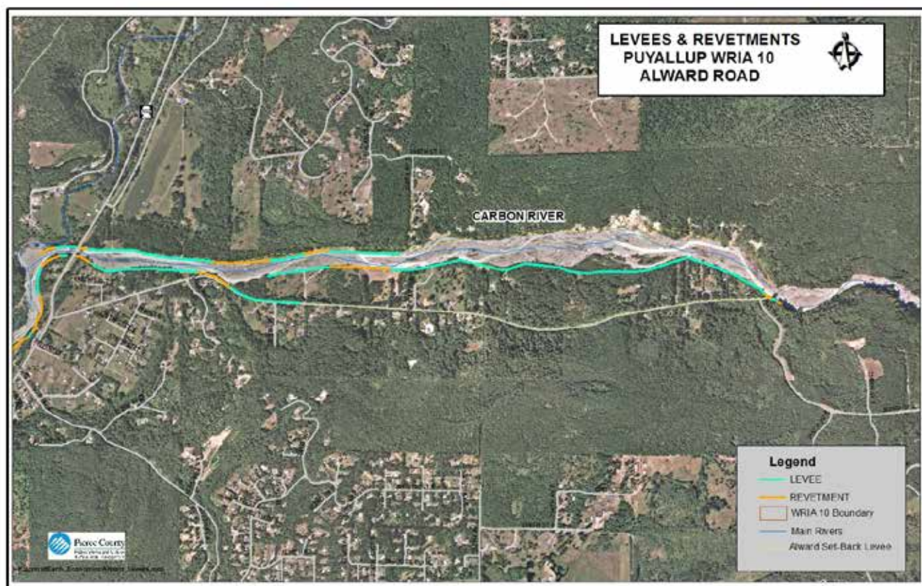
Figure 5: Alward Road Reach Levees and Revetments
