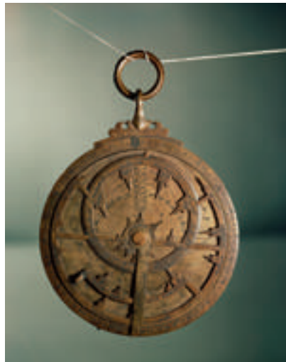
Figure 1 Early astronomers often used instruments called astrolabes to track the positions of the sun and stars.
