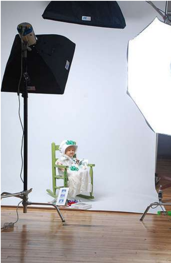
Example of a photographic studio setup: main through a dark umbrella 45 degrees from subject. Fill, using a soft box, almost straight on. Hairlight (softbox) lighting the back of the screen for definition.
