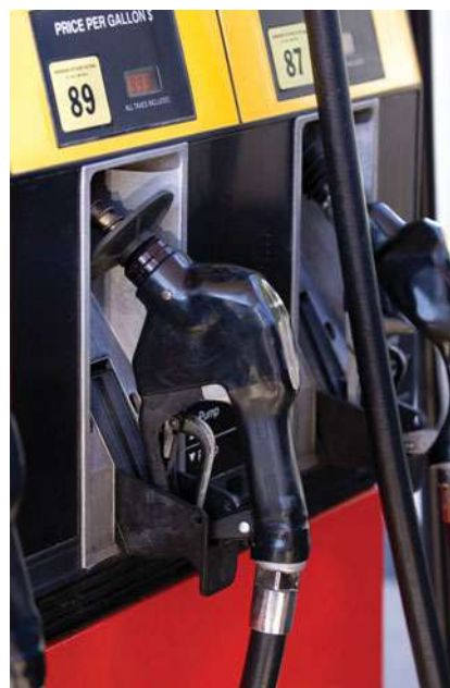
▲ FIGURE 24.6 Octane rating. The octane rating of gasoline measures its resistance to knocking when burned in an engine. The octane rating of the gasoline in the foreground is 89.
