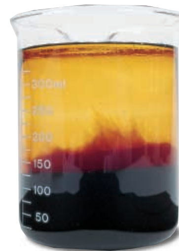
Figure 6.14 The random movement of particles of corn syrup will cause the colored sample to diffuse into the uncolored sample.
