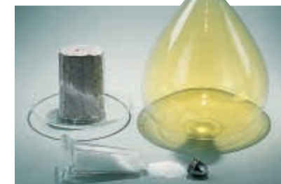
Figure 6.5 Table salt is made from the elements sodium (Na) and chlorine (Cl). The flask contains the poisonous, yellow-green chlorine gas. The lump of silver-white metal is the element sodium. The white crystals of table salt no longer resemble either sodium or chlorine.
