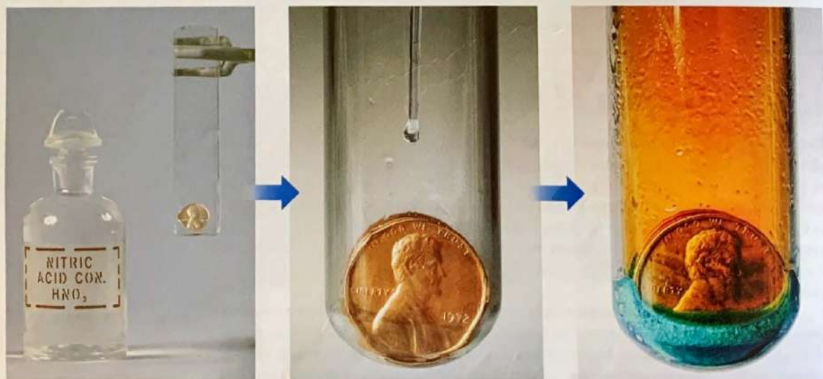
▲ Figure 1.11 The chemical reaction between a copper penny and nitric acid. The dissolved copper produces the blue-green solution; the reddish brown gas produced is nitrogen dioxide.
