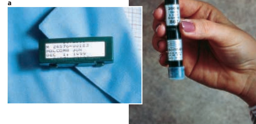
Figure 11.9 Nuclear power plant workers wear radiation badges (a) and pocket dosimeters (b) to monitor their exposure to radiation.
