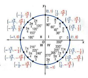
Consider the points on the unit circle for  $\theta = 45^{\circ}$ ,  $\theta = 150^{\circ}$ , and  $\theta = 270^{\circ}$ .
