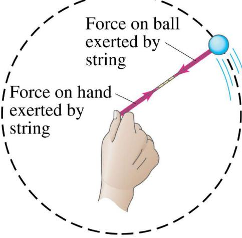
Centripetal force is not a new kind of force. It is a net force. You pull inwardly exerting a force on the ball. The ball exerts an equal and opposite force on the string. This is the outward force your hand feels.
