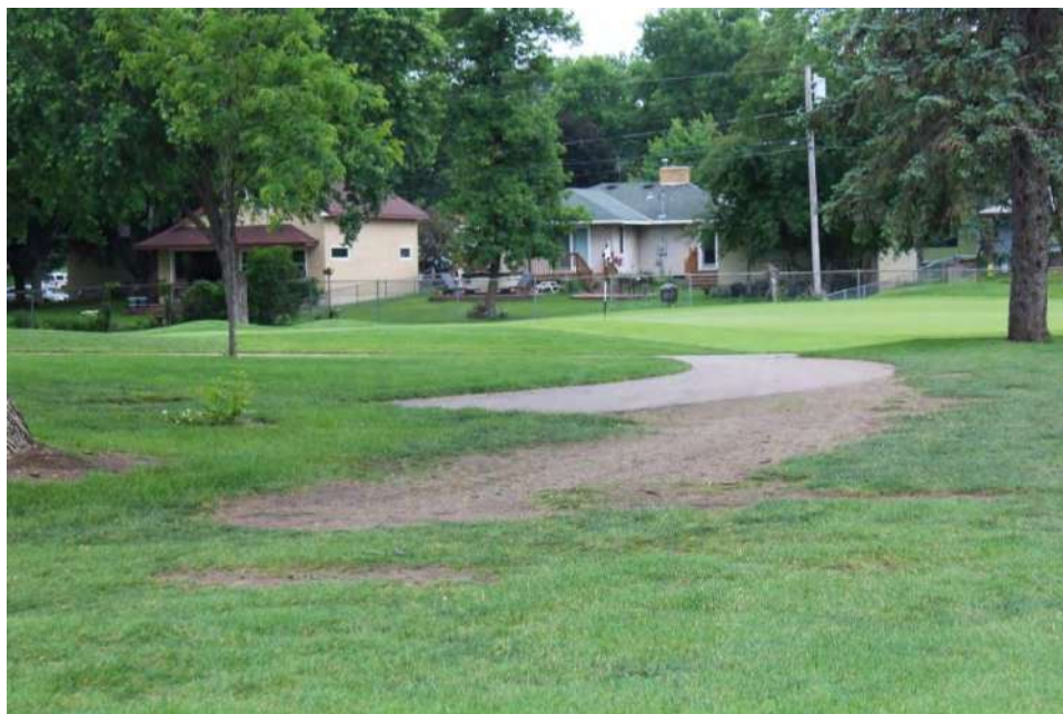
Below – Even if you opt against a full loop system, extending paths further from greens and tees can help reduce wear patterns, if they end on a gentler curve than shown here to spread wear.
