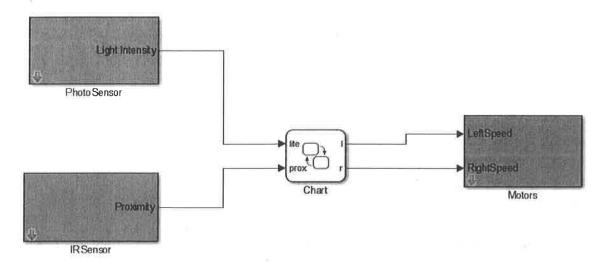
The objective here is to create a robot which follows a hand put up close to it. The combination of close proximity to a hand casts a shadow. The light sensor can be used to figure out if a hand is left or right of the front of the robot depending on a lack of light. The proximity sensor is factored in so the robot following behavior is only present when a hand is close enough.
