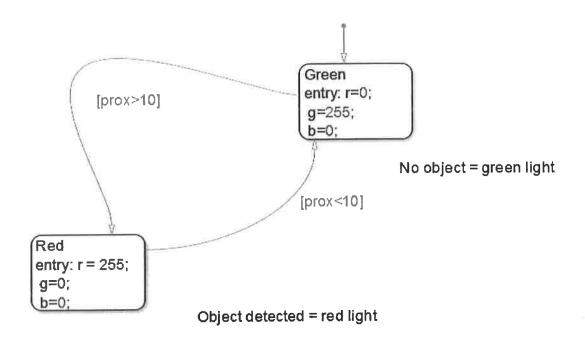
Explanation: The chart flows to different combinations of red, green and blue depending upon the proximity readings from the IR sensor block. The expression of code in a flow chart rather than a function helps aid the process of representing the robot's behavior.
