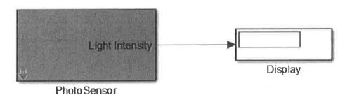
If you run the above Simulink model in external mode you can take readings from the light sensor in the above way. You'll find the "Display" blocks in the "Sinks" tab of the Simulink block builder.
