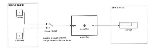
We can adapt the model above. Instead of manual control by way of mouse click. Attach a sine wave Simulink block and connect it to the middle of the switch block. Two constant values, 1 and 5, are branched to the switch block. Observe the values in the display block and why these are the particular numbers displayed. Click into the scope to further investigate.
