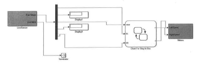
In the chart, SL stands for the leftmost line sensor on the MiniQ robot while SR is the rightmost sensor.
