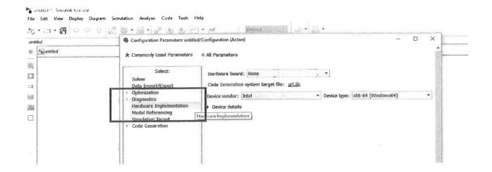
6. You will then need to select the hardware board being used. For our miniQ we are going to select the Arduino Leonardo option as seen in the picture below.
