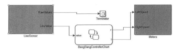
The following model was created to test a "bang-bang" version of line following behavior. The name comes from how the robot dips inwards and outwards towards a line depending upon the light readings taken from the array of five sensors at the bottom of the miniQ robot.
