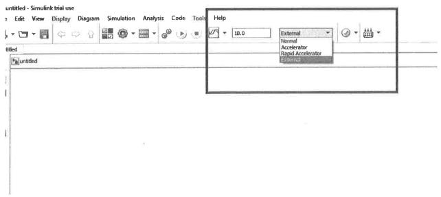
3.In the simulation time frame change the value "10.0" to "inf" as in the picture below. This will allow the simulation target time to run for an infinite period rather than just 10 seconds.
