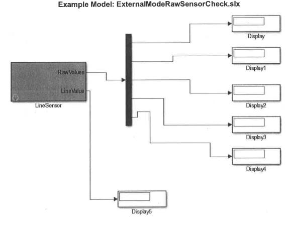
Create the following model and run on your MiniQ robot in "external mode". This will allow you to view the individual sensor readings without going into the serial monitor app. Record the values for each sensor when over black and also when over the color white for later use.
