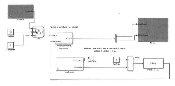
Turning is based on the error
