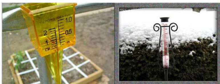
Rain gauge (amount of rain)
