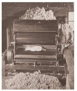
The Impact of the Cotton Gin Whitney's "cotton engine," called the cotton gin [cotton gin: a hand-operated machine that cleans seeds and other unwanted material from cotton] for short, was a simple machine that used rotating combs to separate cotton fiber from its seeds. Using a cotton gin, a single worker could clean as much cotton as 50 laborers working manually [manually: using human effort, not electricity or other power], or by hand.
